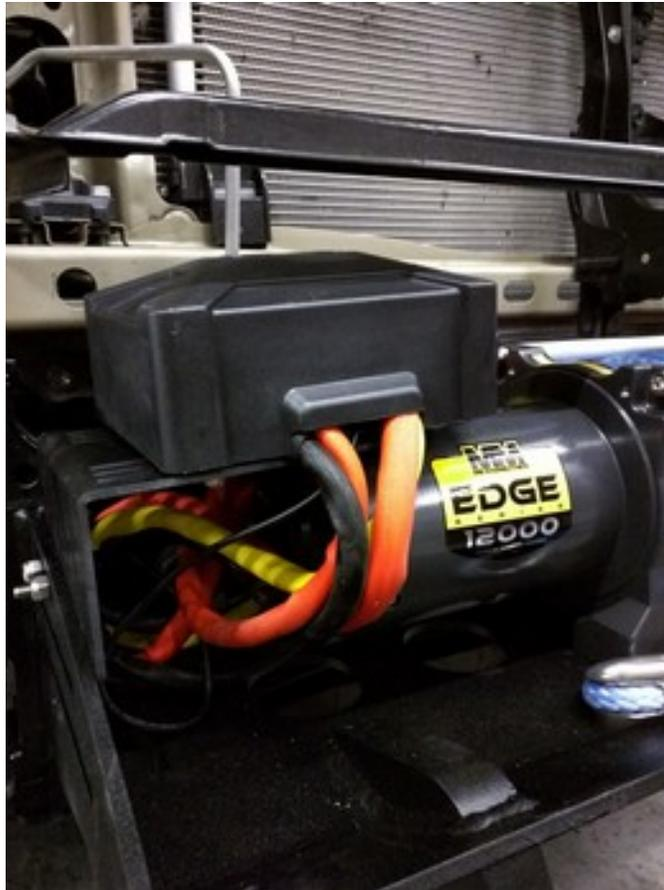
While we used a Mean Mother winch in this photo to illustrate the bracket please note that the control box on Mean Mother winches can mount over the motor side of the winch using factory supplied brackets.
