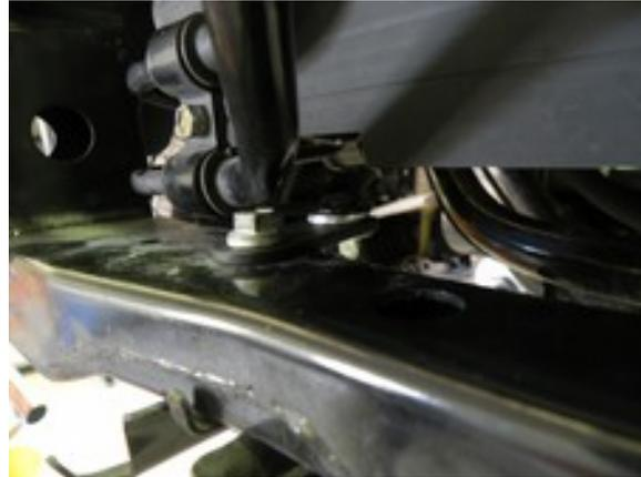
You may also want to loosen the power steering line bracket to help facilitate installing the fasteners on the cooler brackets. Be sure to re-tighten them after you have the cooler moved.
