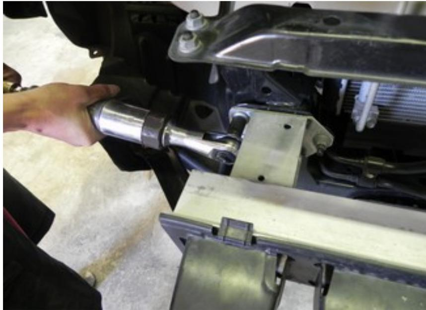
If it is too tight to slide off of the frame studs you can loosen the bolts that attach the tube to the standoffs to release pressure. Pop off the plastic rectangular 'flower pots' from the aluminum bumper tube to expose those nuts then loosen, removal is not necessary.
